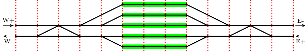
■ Figure 3 The diagram shows 13 columns of “parallel” track segments separated by red vertical lines of the railway station shown in Figure 1.
