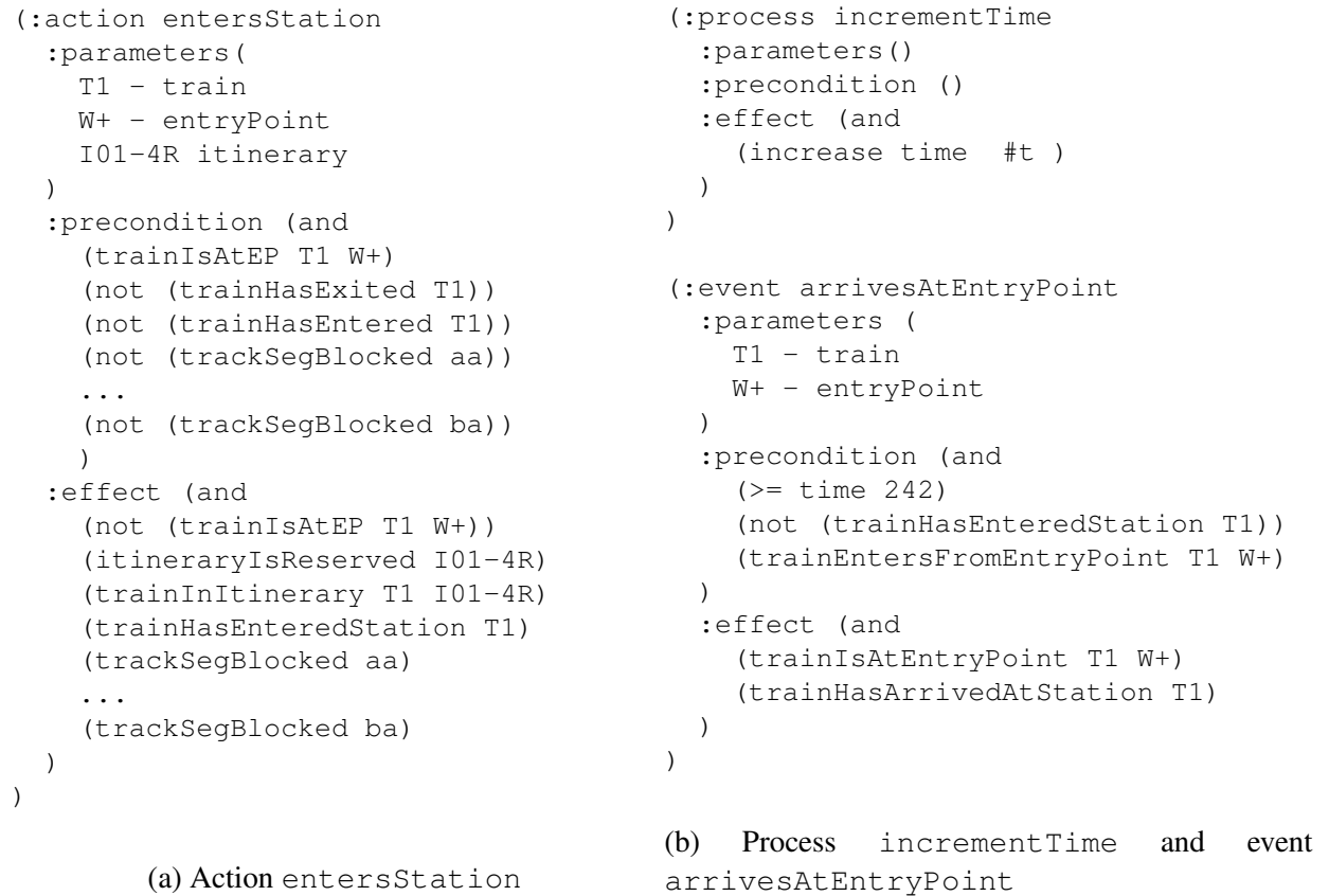
Figure 5.3: The grounded action entersStation which enable a train T1 to enter from an entry-point W^+ through itinerary 01-4R. (right) The process incrementTime which keep track of the flowing of time and the grounded event arrivesAtEntryPoint which signals that a train T1 has reached the endpoint W^+
